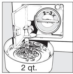
■ Turn the lint trap lid counterclockwise 2 - 3 times. Do **not** remove it. Approx. 2 quarts (2 I) of water will drain out of the hose.
